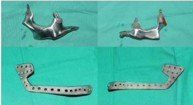
Fig. 1. Customized 3D printed titanium implant: (above: implant for maxilla, below: implant for mandible)
